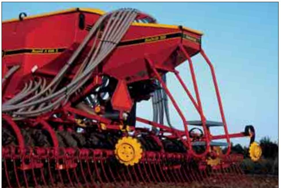
**BioDrill mounted on RDAS.** The large 360 litre hopper harmonises well with the grain hopper on the seed drill. The seed hoses are situated just in front of the Rapid wheels, which cover the seed along with the following harrow.
