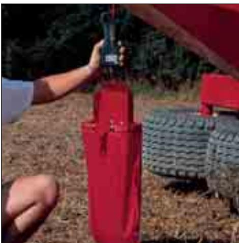
2) The weight of seed multiplied by 100 gives the seed rate in kg/ha. With all Väderstad seed drills, a drilling precision kit is supplied as standard. It includes weighing scales and a test bag – everything needed to carry out a quick and simple calibration in the field.
