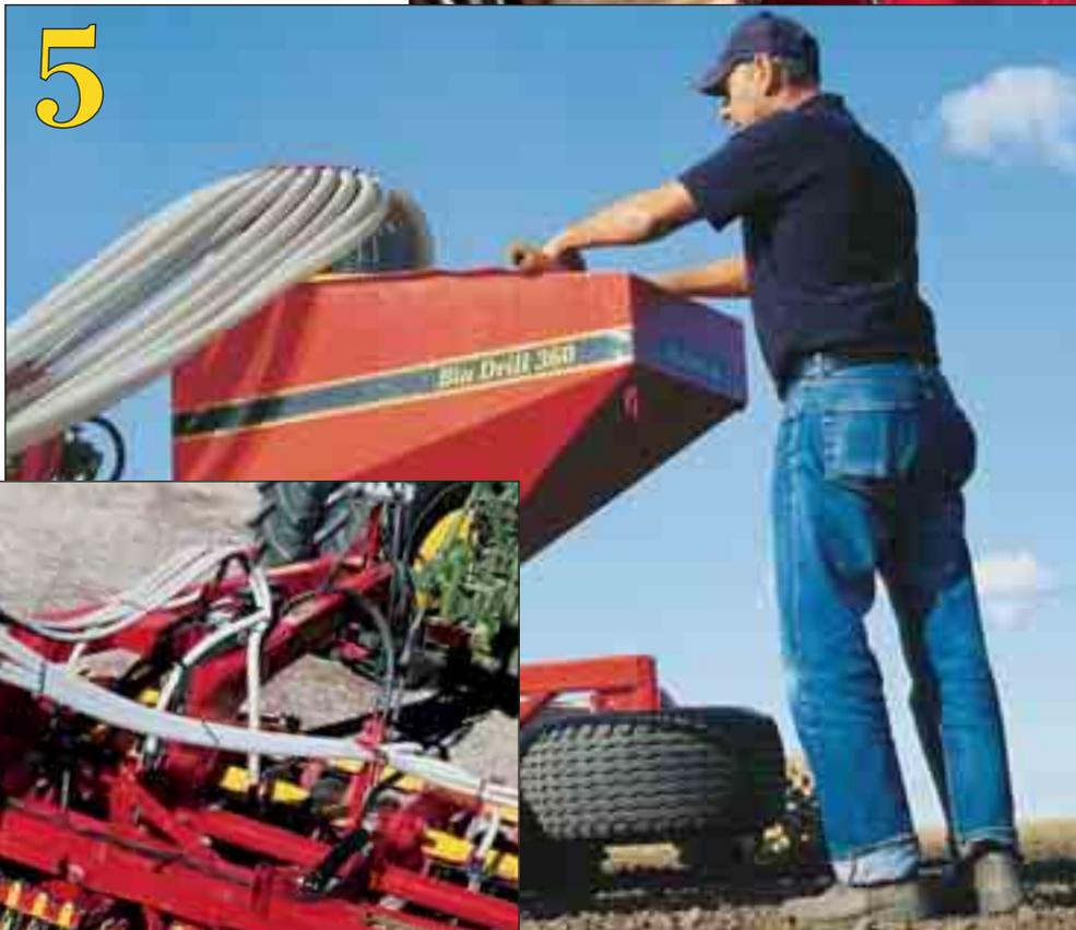
6. The required drilling depth is set before starting and a calibration test checks the amount of seed being metered out. The calibration test only takes an instant.
