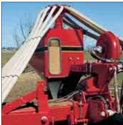
The Fenix system is easy to adjust and the seed rate can be increased/decreased easily even with a full seed hopper. The viewing window on the front clearly shows how much seed is left in the hopper. This means that it can be drilled out down to the last few grams.
