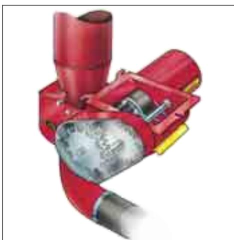
The small seeds are metered out by Väderstad's own tried and tested Fenix system, which allows very precise setting of the seed rate from 1 - 30 kg/ha. It has been shown that the seed distribution produced is very uniform across the entire working width.
