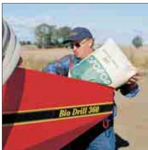
The seed hopper has a huge 360 litre capacity and is placed low for ease of access during refilling. It is also easy to empty out excess seed after drilling. The design of the hopper allows it to be completely emptied.
