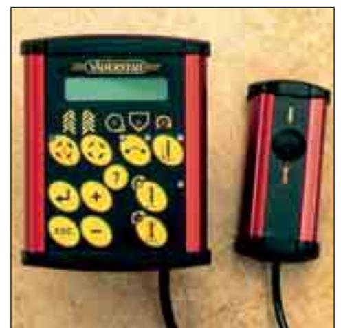
There are two alternatives for controlling the BioDrill: The Control-Switch for switching drilling on or off, or Control Station-Bio (electronic box) which also shows the actual fan rev count and has rotation, tramlining and seed level sensors.
