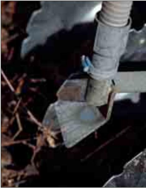
The seed is broadcast by broadcasting plates that distribute the seeds in a uniform spreading arc. The broadcasting plates give the seed a uniform distribution across the entire working width.
